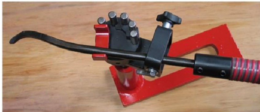
Basic Post Used as Hollowing Rig [with yoke inserted]
